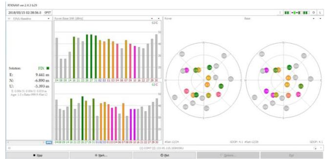
Fig 3. Visible Satellites for Base Station and Rover.
